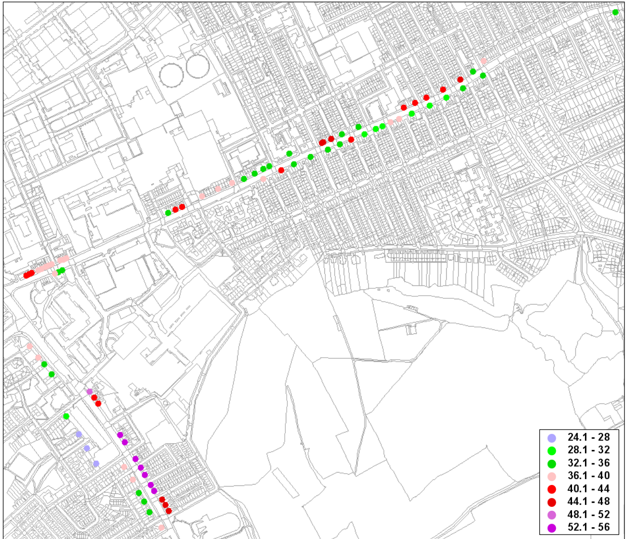
Figure 6 Predicted Concentrations of Nitrogen Dioxide ( \mu\text{g}/\text{m}^3 ) modelled receptors in 2010 within the New Hall Lane study area.
