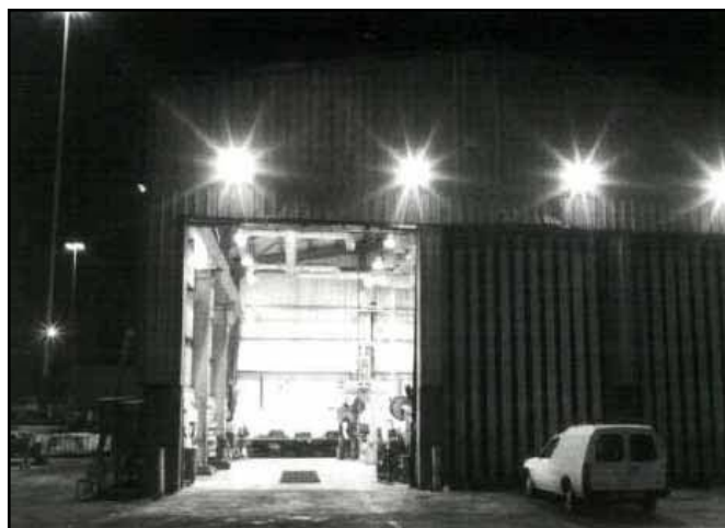
Figure 19 Transition zone between high-and low-luminance areas
