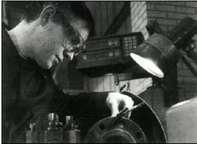
Figure 9 Local lighting providing flexible, directional lighting
