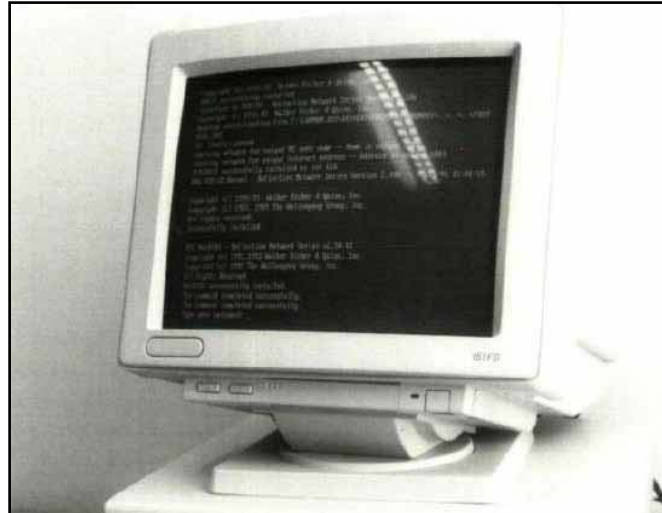
Figure 2 The reflection of a window is masking information on the screen
